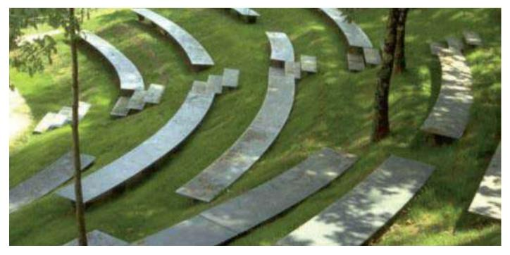
In order to facilitate the use of the amphitheatre as a performance and outdoor classroom space seating will be reintroduced to the embankment in this location. The seating will be prefabricated and detailed to avoid any damaging excavation.
