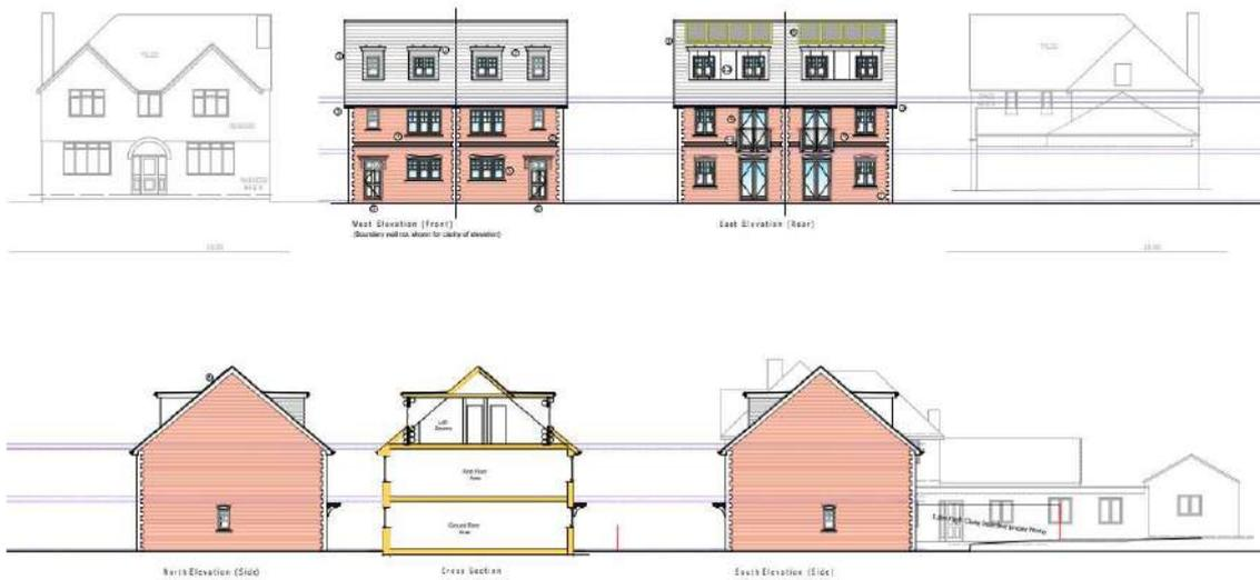
Floor Plans: 4-bed (or 3-bed with first floor "lounge"). Flat roof dormers front and back, solar panels above rear dormers.
